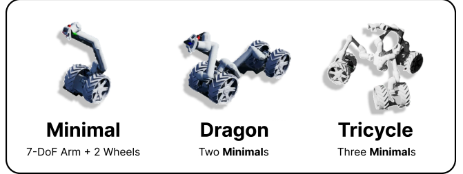
Fig. 1. Three morphologies of the modular robot Moonbot: Minimal (left), Dragon (middle), and Tricycle (right). These diverse configurations pose challenges for reinforcement learning policies to generalize effectively across morphologies.
